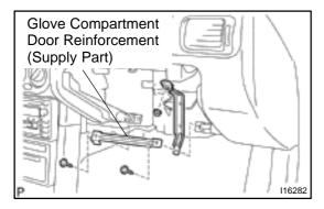
(d) Install the glove compartment door reinforcement (supply part) and No. 1 instrument panel lower bracket with the 2 screws and nut.
